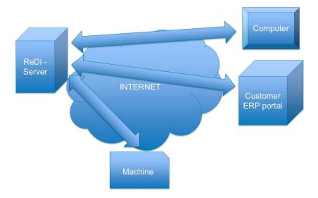
ReDiService is a machine side telematics solution for mobile machines built around Exertus control system.
