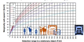
Figure 7 Radar (blue) and lidar (orange) detection ranges to the various objects analysed in this study, and safe stopping distance from different speeds with varying tyre-road friction coefficient. The delay t<sub>d</sub> (see equation 2) from the first obstacle detection to the beginning of emergency braking is assumed to be 0.7 seconds.
