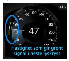
Connected Traffic Signals in Gothenburg, Stockholm and Uppsala. The use cases being tested are Time To Green (TTG), Green Light Optimal Speed Advisory (GLOSA) and Traffic Signal Priority for designated vehicles. The goal with connected traffic signals is to increase the capacity in the intersection.
