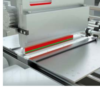
back lining station
