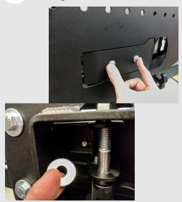
Put the latch handle plate and the carriage bolts in place on the latch. On the back side of the latch, you can access one of the bolts. Put a washer and a nyloc nut onto this bolt.
