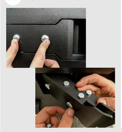
Adjust the latch handle plate so that it has an even reveal with the cutout in the swing arm.
