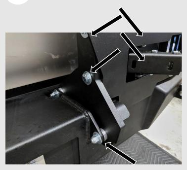
Loosen the 4 carriage bolts (two on the side and two on the back, indicated with downward-pointing arrows) so the latch can slide up and down on the arm.
