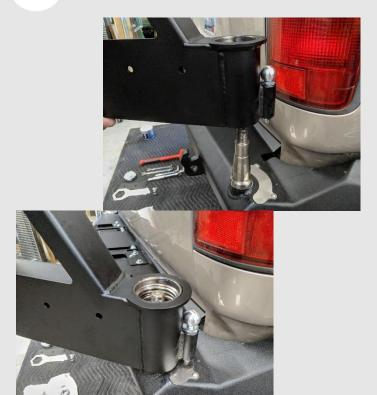
Carefully lower the swing arm onto the bumper spindle; be sure not to damage the seal.
