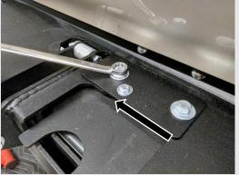
Loosen the three bolts on the bumper latch plate (the plate on the same side as the swing arm). The four bolts on the latch assembly should still be loose from earlier.
