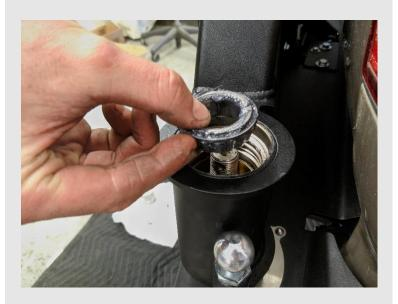
Drop the smaller bearing onto the spindle. Wiggling the arm around a little bit while doing this can help seat the bearing.
