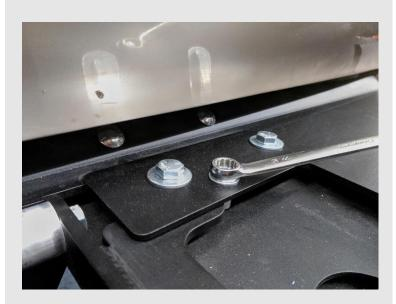
Snug the three bolts on the bumper latch plate. Be careful not to over-tighten and strip the center bolt especially.
