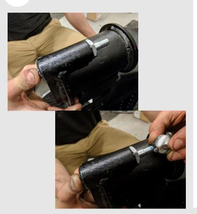
Press in the bottom of the lockout plunger, then hold it in place while you unscrew and remove the nut, exposing the threads.
