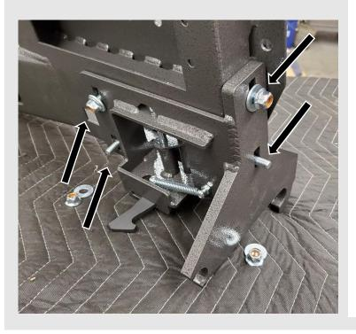
Insert the two long carriage bolts through the side interlock plate (downward facing arrows) and the two shorter bolts into the slotted holes in the front handle (upper facing arrows). Washers and flange nuts can be installed.
