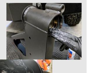
Apply some grease around the interior seal surface and the thread on the swing arm, as shown.
