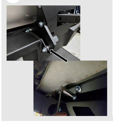
Close the latch on the swing arm and check how much play there is. If the latch has wiggle room, you can try tightening the latch adjustment bolt more, but it might require some trial-and-error of sliding the latch plate slightly forwards or backwards and testing the fit.
