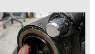
Apply some grease to the interior of the seal.
