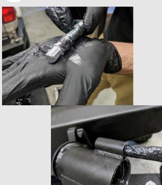
Apply some grease to the large cylinder on the lockout plunger, as well as its corresponding hole on the swing arm.
