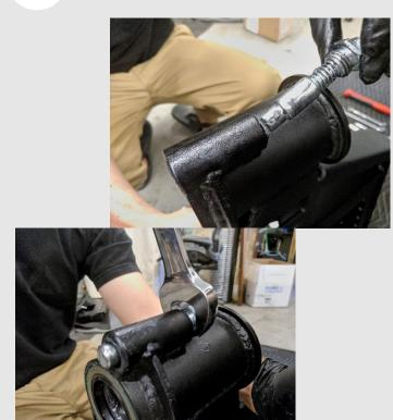
Liberally apply anti-seize to the pull pin assembly, including the threads of the plunger nut.
