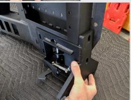
Open the latch box and retrieve the latch and hardware pack. Sort out the short and long 3/8" carriage bolts, there should be two of each.
