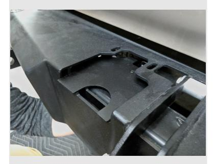
Slide both of the lower latch plates into place from underneath the bumper. Pictured is the correct orientation for the left side latch plate; the right side plate is a mirror image of the left.
