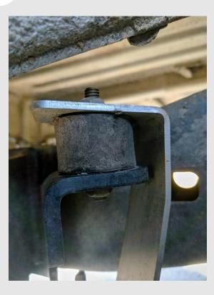
On the right side forward bracket, there is a tab above the exhaust. Insert one of the rubber isolator's posts into this tab from the top, and put the exhaust hanger onto the top post so that it hangs down, as shown.
