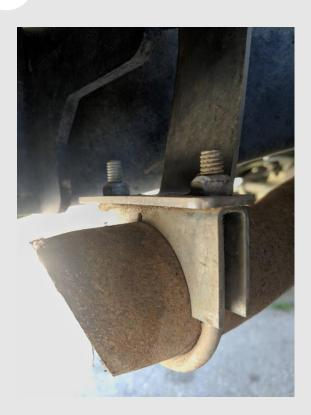
Fasten the included u-bolt around the exhaust pipe and insert the u-bolt's rods through the slotted holes in the bracket. Then use the remaining two torq nuts (with washers) to tighten the u-bolt clamp down. At this point, you can torque down these nuts as well as the ones securing the exhaust hanger to the forward bracket.
