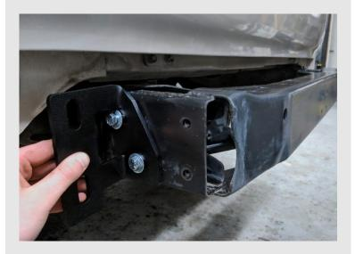
Sandwich the frame between the driver side internal frame plate and the driver side rearward bracket (pictured).
