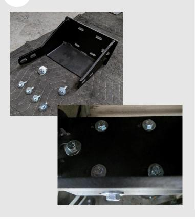
Start the four M8 bolts and the 3/8" bolt on the side of the bracket, as well as the M12 bolt on the bottom of the bracket.
