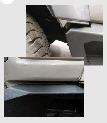
The bumper will have some movement forwards and backwards. Adjust it so that it aligns with the fender well on each side, while also centering the bumper left/right. Then adjust the frame brackets to sit flush with the mounts on the bumper.
