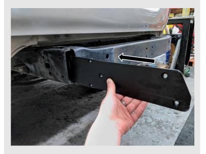
This plate needs to slide inside the frame rail. This might be tricky as there are nuts welded to the inside of the frame from the factory.
