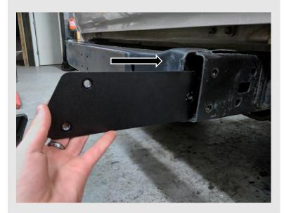
The right side plate should be much easier to install, just slide the plate in until the holes are aligned and set it flush against the inner right wall of the frame rail.
