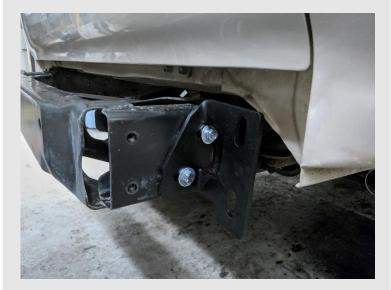
Using the two rearward most holes in the internal frame plate, start two 3/8" bolts.
