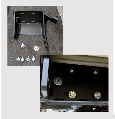
Start the four M8 bolts and the 3/8" bolt on the side of the bracket, as well as the M12 bolt on the bottom of the bracket.
