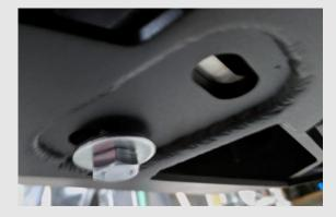
On each side, slide a spacer in between the frame and the mount on the bumper.
