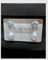
Put the Delta name plate over the four holes in the center of the bumper, and insert and tighten four M12 bolts into the holes. The top two are shorter and will thread directly into the frame, while the bottom two are longer and need nyloc nuts, reachable from the inside of the bumper. Tighten them all down to 99.6 ft-lbs (135Nm).
