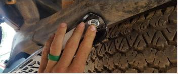
Install the yellow chromate 3/8" bolt with a yellow chromate washer and pivot the bracket into the frame crossmember.
