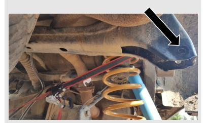
Remove the Panhard axle bolt on the frame side.
