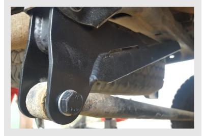
Install the Panhard into the remaining saddle of the drop bracket and bolt in with provided M12 hardware.
