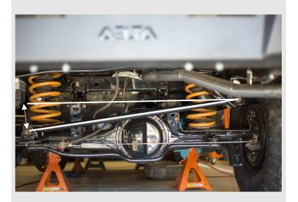
Before working on the vehicle, lift the vehicle a few inches and put jack stands under the frame towards the rear of the vehicle, the wheels should remain in the ground.
