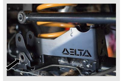
Remove the bolts and single washer from the DELTA bracket and set them aside. With the panhard link lifted out of the way, position the lift bracket into the original axle link point and around the upper left 4 link brace.
