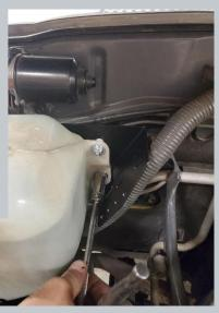
Replace the two hinge panel bolts and tighten them back down over the bracket. Then tighten the rightmost M8 bolt (which will be much easier with a socket extension, as shown), and then finally the bottommost M8 bolt. That bottom bolt is tricky to access; you may have more luck with a ratchet box wrench.
