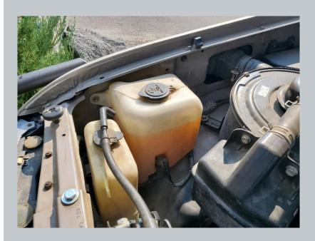
Disconnect and unbolt the washer fluid tank so you can remove it from the vehicle. Be prepared either to drain the tank or to quickly plug the hole (we used a piece of hose with a bolt in the end).
