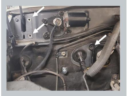
There are three more bolts to remove, notated with arrows. The rightmost (from the camera's perspective) bolt will be replaced, but the two on the hinge panel will be reused, so don't lose them!
