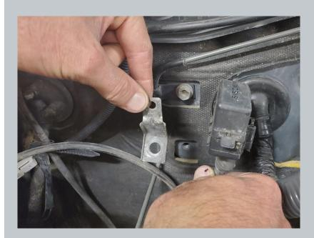
The stock diagnostics port is mounted to a small bracket on the passenger side firewall. The port should unclip from the bracket, which you can then detach by undoing the M8 bolt. This bolt will be replaced by hardware from the kit, so you can set it aside.
