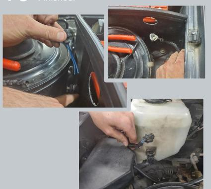
Trim off the stock wiring harness a few inches below the connector, as shown. Using the included wire, heat shrink butt splices, and braided loom, extend the harness so it can reach the fluid tank in its new location. Be careful not to accidentally reverse the polarity.
