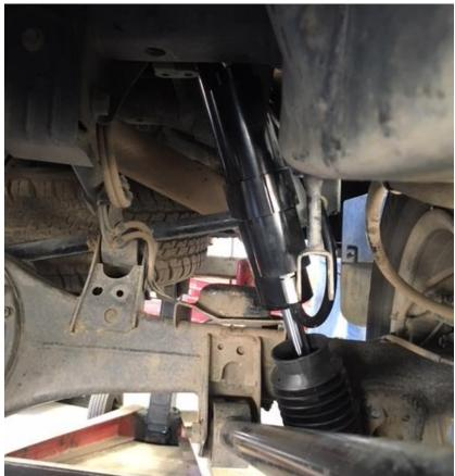
Reservoir is slightly outward towards the chassis rail to clear sway bar with the hose.
