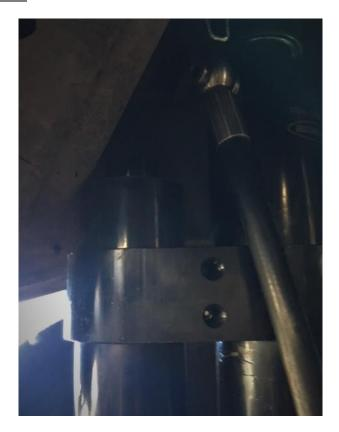
105 Series Pictured with short hose to the reservoir. Make sure the reservoir is as high as you can and clears the sway bar at the bottom through all travel. Note it is slightly off to the chassis side of the shock. It should not foul on the lower trailing arm.
