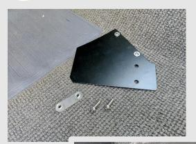
With the same process as the passenger side plate, attach the driver side plate to the shifter console with two button cap screws. Again, leave them loose enough for the plate to move relatively freely.
