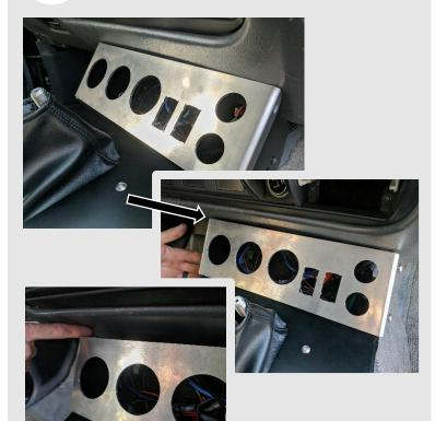
Place the gauge/switch mount faceplate over the two side plates, and lightly thread four button cap screws through the side holes and into the side plates.
