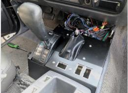
Using the same 90° angle as when you removed the stock console, lower the custom one into place.
