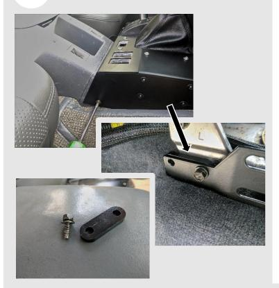
Using three of the four Phillips head screws from earlier, secure the custom shifter console into place and tighten them down. For now, do not install the forwardmost screw on the passenger side.
