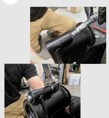
Push the lockout plunger into the hole on the swing gate and snug it down with a 7/8" wrench.
