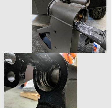
Apply some grease around the interior seal surface and the thread on the swing gate, as shown.
