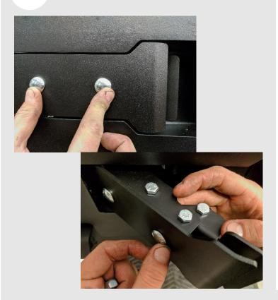
Adjust the latch handle plate so that it has an even reveal with the cutout in the swing gate. Then open the latch (while holding this plate in place) so that you can put a washer and nyloc nut on the other carriage bolt, and tighten it down. Close the latch handle so that you can check if the reveal is still even, and make adjustments if needed.
