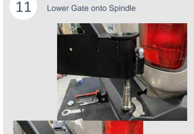
Carefully lower the swing gate onto the spindle on the bumper. Do not close the gate.
