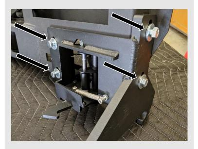
Insert four of the provided inchlong 3/8" bolts with washers into the four holes mounting the latch to the gate, as shown. Only finger tighten them for now; they should be loose enough for the latch to slide up and down.
