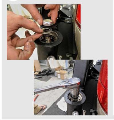
Install the washer and nyloc nut onto the spindle on top of the bearing, and tighten it down until the bearing is snug.
