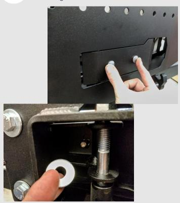
Put the latch handle plate and the carriage bolts in place on the latch. On the other side of the latch, you can access one of the bolts. Put a washer and a nyloc nut onto this bolt.
