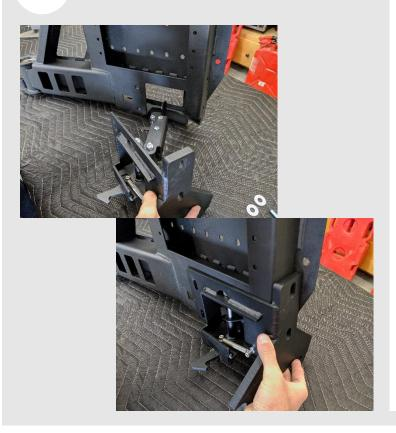
Insert one of the latches into its place on one of the swing gates. Note that the left latch is only compatible with the left swing gate and vice versa, so if it doesn't fit, try the other latch (or the other swing gate).
