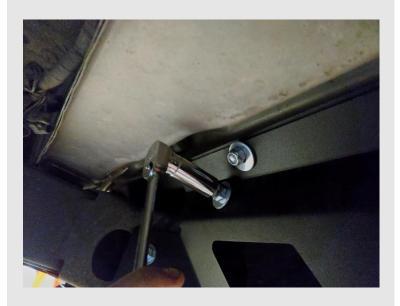
Under the bumper, you can access the latch adjustment bolt. Tightening this bolt draws the latch post towards the front of the vehicle, which sets the latch strike distance.
