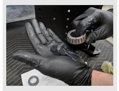
Using either a bearing packer or your own two hands, thoroughly pack both bearings with grease.
