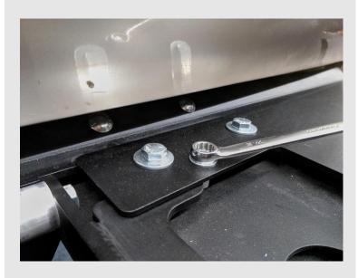
Snug up the three bolts on the bumper latch plate. Be careful not to over-tighten and strip the center bolt especially.
