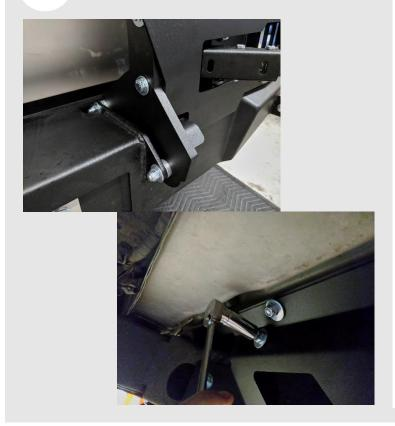
Close the latch on the swing gate, and see how much play there is. If the latch has wiggle room, you can try tightening the latch adjustment bolt more, but it might require some trial-and-error of sliding the latch plate slightly forwards or backwards and testing the fit.
