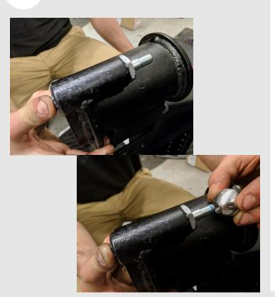
Push in the bottom of the lockout plunger, then unscrew and remove the nut, exposing the threads.
