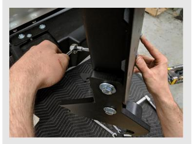
Using a 1/2" socket on an extension, tighten down the first carriage bolt to 13 ft-lbs (17.6Nm) with the latch handle closed and the handle cover centered in the hole.
