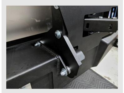
Lift up the latch assembly in the swing gate and slowly close it, guiding the clevis plate onto the dowels on the bumper.
