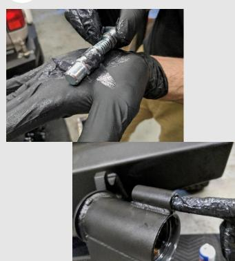
Apply some grease to the large cylinder on the lockout plunger, as well as its corresponding hole on the swing gate.
