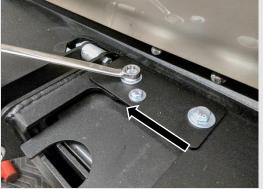
Loosen the three bolts on the latch plate on the bumper (the plate on the same side as the swing gate). The four bolts on the latch assembly should still be loose from earlier.
