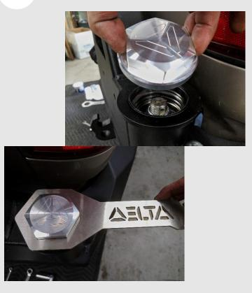
Install the cap onto the swing gate's hinge. Make sure that the o-ring in the cap is seated evenly, and then use the provided cap wrench to snug it down until flush. Careful not to overtorque, flushing the cover and snugging it is adequate.
