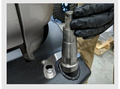
Finally, grease the swing gate spindle on the bumper itself.
