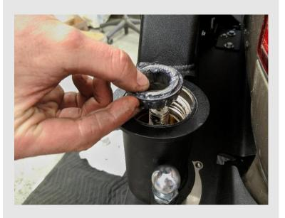
Drop the smaller bearing onto the spindle. Wiggling the gate around a little bit while doing this can help seat the bearing.
