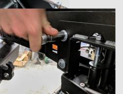
Once you have the latch adjustment bolt initially set, snug up the two accessible latch assembly bolts on the swing gate. Then carefully open the latch all the way to the second stage and open the gate, so that you can snug the other two latch assembly bolts.
