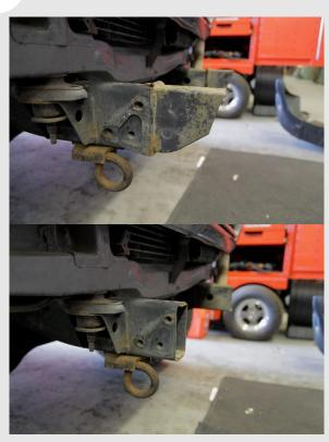
Later models of the Landcruiser and LX450 will have these frame extensions hanging on the ends of the frame rails
