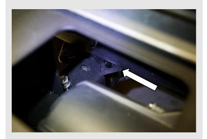
Take the shims removed from a given side and insert them into the gap between the top of the frame and the bumper mount.
