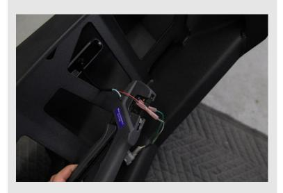
Crimp the unused end of the butt connector to the turn signal wire on the Delta bumper
