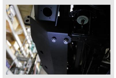
Start the remaining four (rearward) M12 bolts holding the bumper to the frame.
