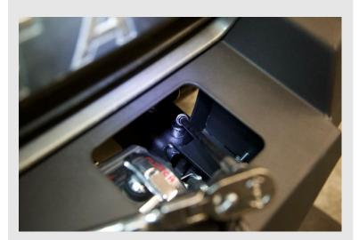
The two forward top bolts can be reached with one long extension and a 19mm swivel socket.
