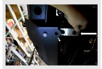
Insert as many shims as will fit into the gap between the bottom of the frame and bumper mount (on each side).
