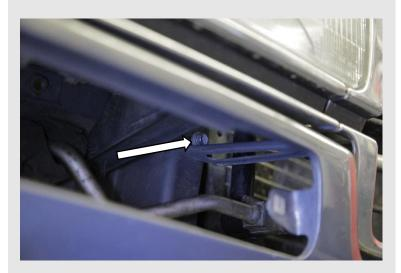
With a short 10mm socket, remove the two bolts (1 per side) holding the lower panel to the core support.
