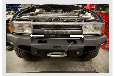
Note the size of the gap between the bumper and headlights.
