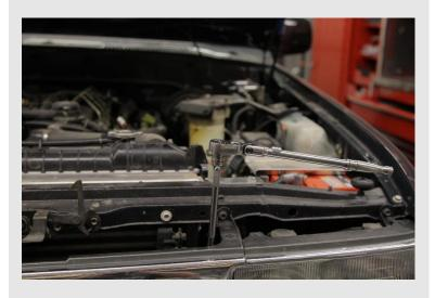
The rearward top two bolts can be reached with two long extensions and a 19mm swivel socket.
