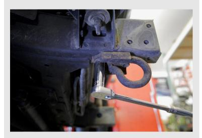
With a 17mm socket, remove the two bolts that hold the factory shipping tie-downs to the bottom of the frame.
