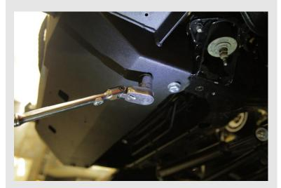
With a 19mm socket, tighten all four of the bottom bolts first.
