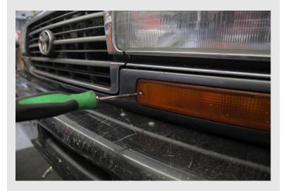
With a Phillips screw driver, remove the screws that hold the turn signal in place.
