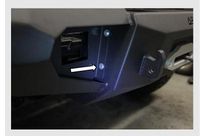
If you choose to add auxiliary light using the light mounts in the Delta bumper, it should be noted that there is a slotted bolt hole in the light mount, allowing for the light beams to be aimed as desired.
