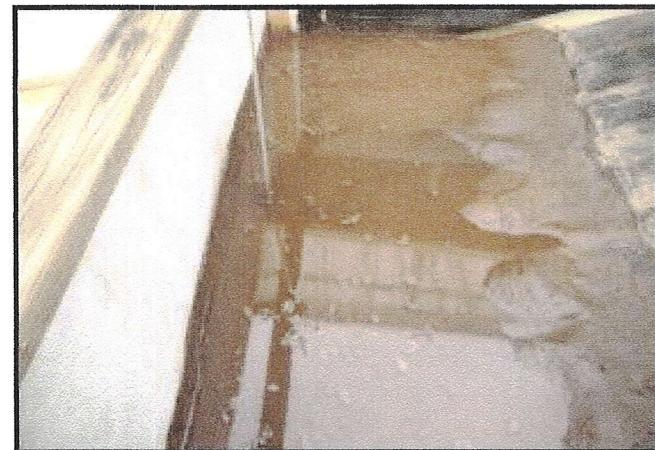
Downstream seepage after runoff stops / Retained sediment at end of test
