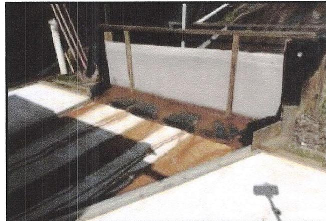
Runoff introduced for 30 minutes / Seepage and ponding monitored for up to an additional 60 minutes.
