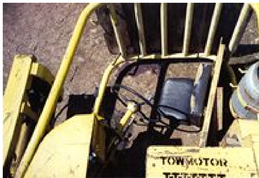
Photo 2. Overturned Forklift – Unsecured Operator's Seat
