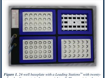
Figure 1. 24-well baseplate with a Loading Stations™ with twentyfour loading posts in the upper right well. The remaining three wells each have HT BioFlex® culture plate in blue, rubber gaskets sitting atop a 24-well Loading Station™.
