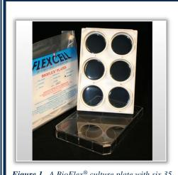
Figure 1. A BioFlex® culture plate with six 35 mm wells and silicone elastomer well bottoms.
