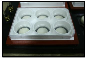
6. Set the Plexiglass sheet on top of the culture plates. Apply weight to the top of the Plexiglass sheet, 5 to 10 lbs is recommended.
