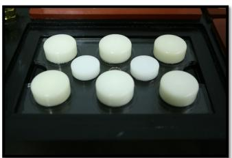
3. Apply a liberal amount of silicone lubricant to the top and top edges of the six Loading Posts. Ensure you reapply lubricant before each experiment.
