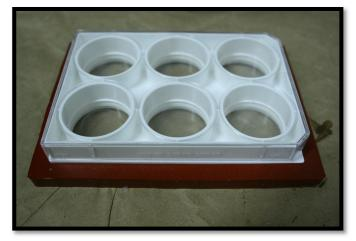
5. Insert the culture plate with rubber gasket into the baseplate, directly over the Loading Station. Ensure that the gasket is pressed firmly into the baseplate.
