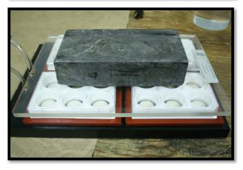
Plates are now ready for tension application. Please see the Tension User Manual for further instructions on applying strain.
