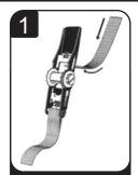
Open ratchet handle flat and insert end of strap through opening
