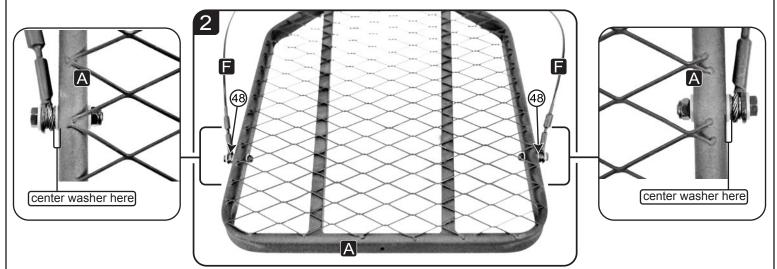
Attach one end of each Platform Support Cable to either side of the Foot Platform A using 2-M8x45mm bolts with 3 washers (as shown Above).
