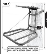
STEP 5: Wrap Tree Buckle strap J around the tree once and insert the strap through the buckle. Pull excess strap to tighten.
