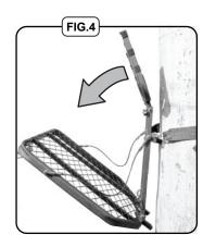
STEP 4: Unfold the stand by bringing the platform downward (See Fig.4) Pull seat platform downward and adjust seat.
