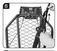
Insert the tag end of the Backpack Strap & through the loop end of the Backpack Strap &.
