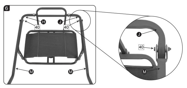
Attach Shooting Rail Arm M to Left and Right Armrest Armrest and Jusing 1-M6x40mm Bolt with spacers 40 for each side.
