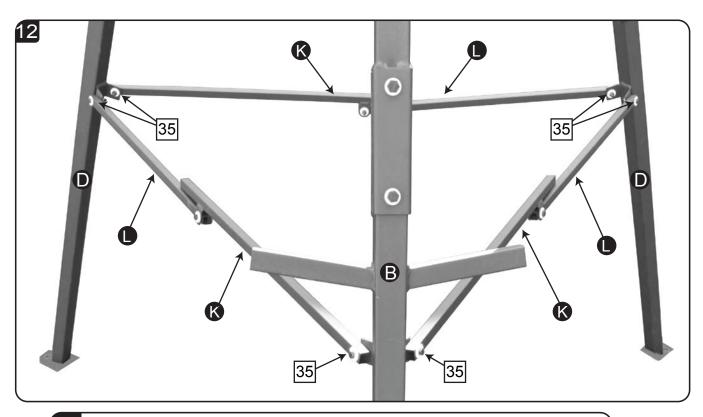
Attach Assembled Cross Braces to the outside of each bracket on Leg Sections **12** Bottom Ladder Section **B** using **1-M6x35mm Bolt 35** at each point.
