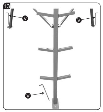
Insert Ground Stake **v** through hole on foot of each leg when the stand is in the desired position.
