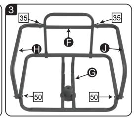
Assemble each Cross Brace to each Cross Brace with Bracket using 1-M6x35mm Bolt 55 Set aside for future use.
