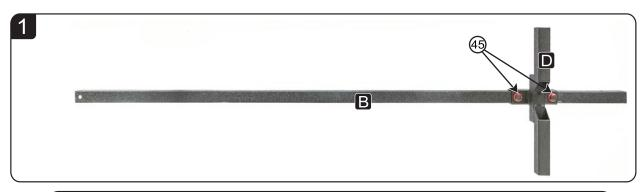
Slide Center Attachment Bracket onto lower end of Ladder Stabilizer Outer Bar connection holes, attach using **2-M8x45mm bolts** 45
