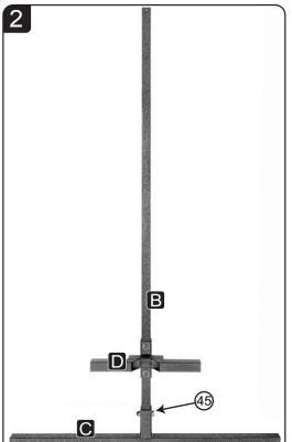
Slide Ladder Stabilizer Outer Bar B assembly onto Stabilizer Base C. Attach using 1-M8x45mm bolt
