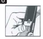
To release tension, push spring loaded retaining lock and simultaneously pull on strap
