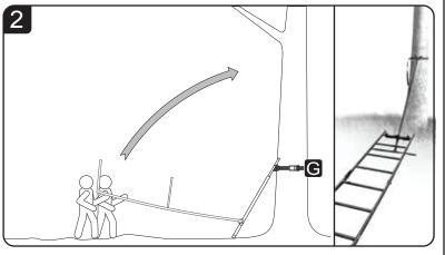
Once the ladder stand has made a firm contact with the tree, check sturdiness of connection. Check that it is securely leaning in place with both hands on the ladder rails.
