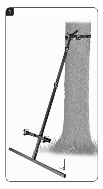
Follow your ladder stand manufacturer instructions in locating an appropriate tree. Finding as level ground as possible, lean the Ladder Aid Stabilizer assembly against the tree so that the Ladder Attachment Brackets are facing OUTWARD. Adjust the Inner Stabilizer Bar to a correct height and leaning angle to work best with your ladder stand.
