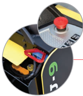
Battery disconnect lever and emergency switch
