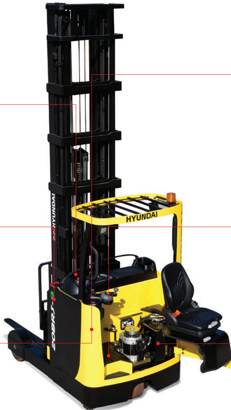
Battery disconnect lever and emergency switch
