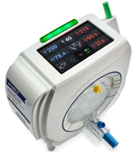
The Nautilus™ Module connects to most component-based blood pumps. Blood enters the device and passes through both the heat exchange membrane—where temperature is adjusted—and the gas transfer membrane—where oxygen is added, and carbon dioxide is removed. The device contains integrated sensors with an electronic touch screen display and a status bar that enables vital, at-a-glance monitoring of hemodynamic device health parameters.
