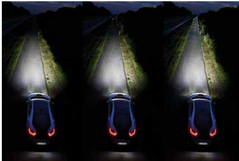
Picture 2: High-Beam Laser-Light Booster in BMW i8
