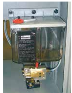
MQL Microlubrication system. Available for all series.
