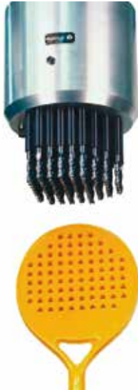
Simultaneous drilling of 76 holes in a paddle pallet.
