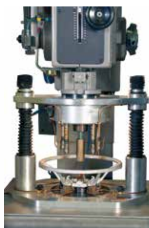
Multi-spindle headstock drilling detail of car handwheels.
