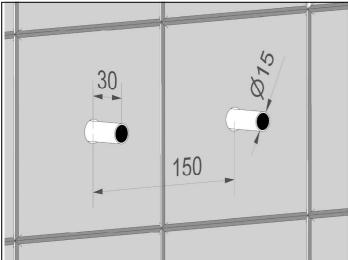
Ensure existing 15mm copper supply pipes are at 150mm centres and protrude from the tiling surface by 30mm.
