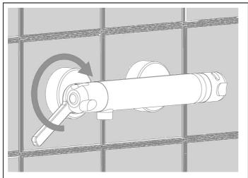
We recommend that the pipe work is well flushed through before installing the bar shower mixer to prevent debris damaging the mixer.
