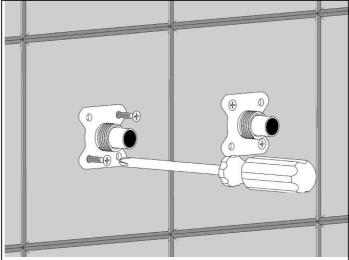
Offer up the brass brackets, ensure they are square and level, mark and then drill holes in the tiles or wall surface with a suitable drill. Insert wall plugs to suit the screws you have chosen (not supplied). Fix the brackets in place with at least two screws in each (preferably four in each).
