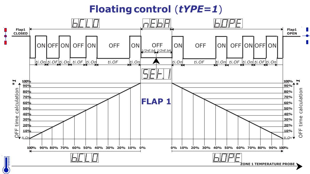
\*<sup>1</sup> When the system operates in Floating proportional mode, the ON working time is fixed ( $ti.On$ ), while the OFF time starts from a maximum setting ( $ti.OF$ ) and is gradually reduced according to the cold and hot band width ( $b.CLO$  and  $b.OPE$ ).
