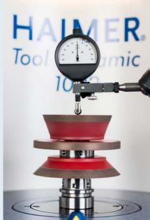
Runout measuring device
