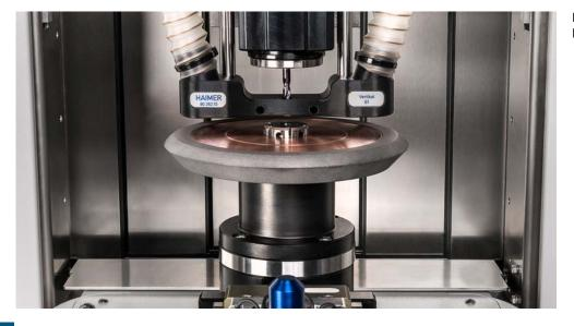
Balancing of grinding wheels by axial drilling
