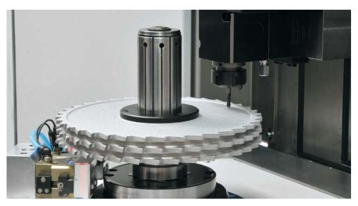
Balancing of PCD jointing cutters for laminate Balancing enables the best edge quality for the piece of furniture by vibration-free tool run. In addition the noise while machining is
