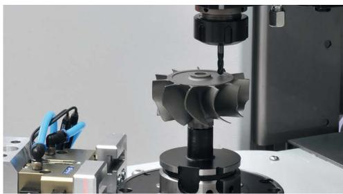
Compressor wheel for turbo charger Axial drilling.
