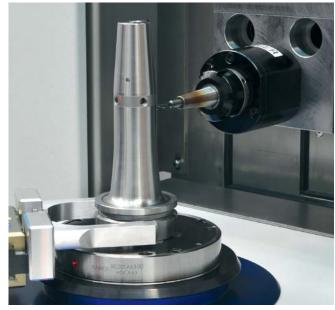
Automated correction of unbalance via CNC machining unit
