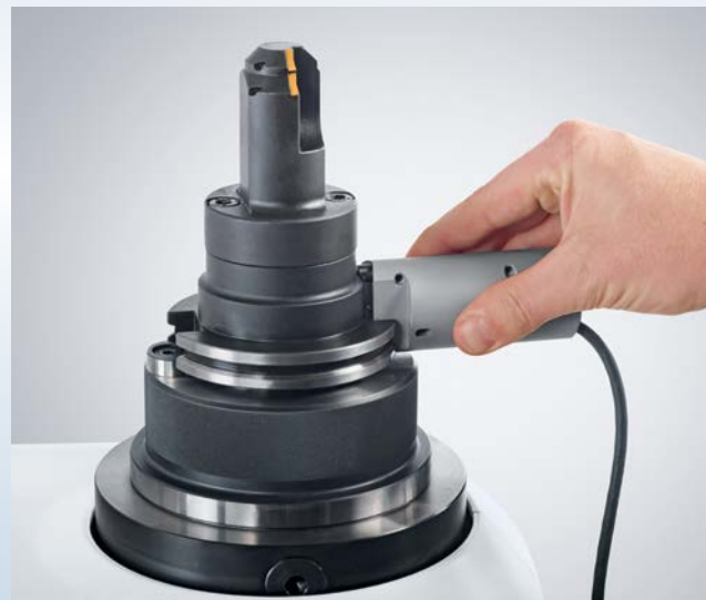
Manual positioning of the read/write head
