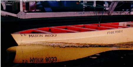
Comparison of wave pattern. MARIN model tests/GD CFD calculations
