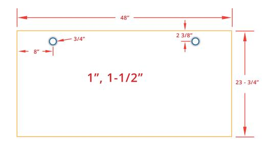
Cardinal Acoustics uses a section of 3/4" o.d., 1/2" i.d. PVC pipe for 1" and 1-1/2" baffles. PVC is inserted in 3/4" holes located as shown.
