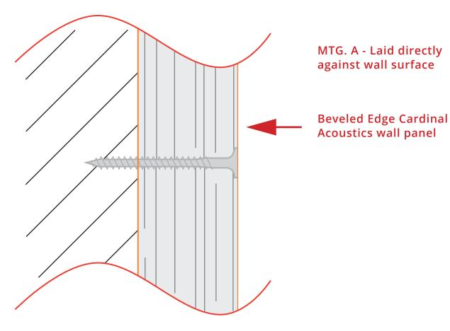
Cardinal Acoustics painted drywall, self-tapping and tapcon screws should be used on all applications.
