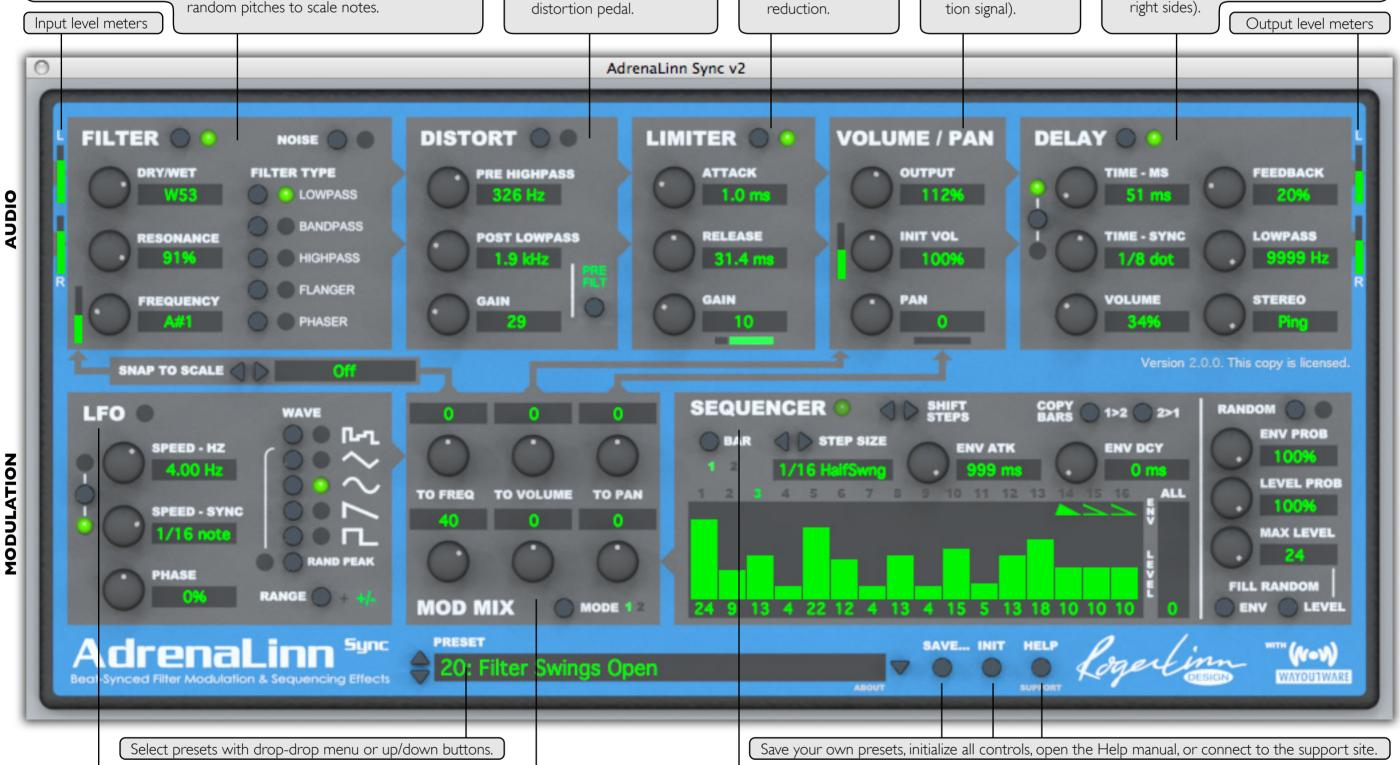
LFO -- A Low Frequency Oscillator, used for modulating the filter frequency, volume or pan with
