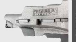
PCD brazed tipped, steel or solid carbide besed body adding chipbreaker control, allows you to improve chip evacuation increasing the productivity as well as a higher tool life. Recomended In particular for materials producing long chips, such as aluminium wrought alloys with low Si conten
