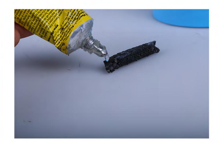
4. Spread some UHU POR on the piece of bumper that broke off
