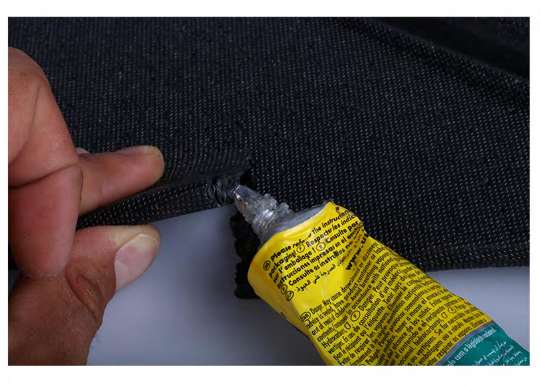
3. Spread UHU POR glue on both side of the crack
