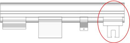
• The final solution would look something similar to the picture below on the standing seam roof. The number of raceways needed would be dependent on the roof layout.
