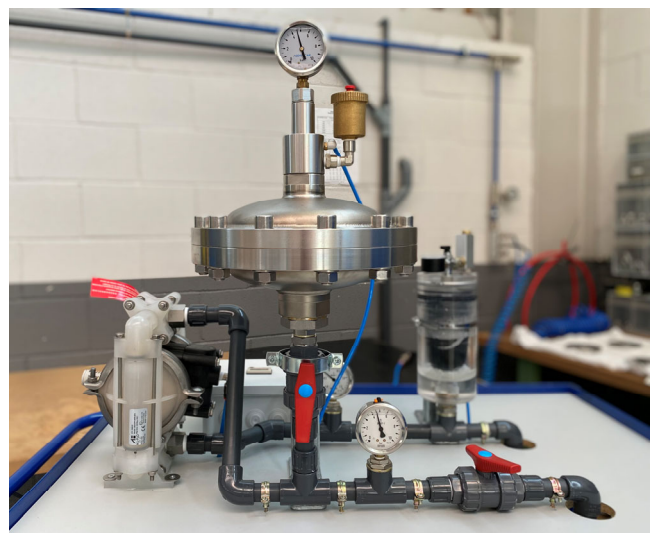
Picture: Active dampener cycling test for durability verification
