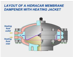
If the installation of heating liquid is not available in the process, we can also provide the dampeners with an external envelopment of heating resistors.
