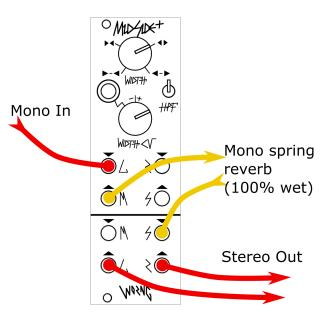
This classic patch comes from the ARP 2600, which creates a wide reverb effect using Mid/Side processing. Patch your mono signal to the Left input and then take the Mid out and patch to a spring reverb. Return the 100% wet reverb to the Side input and monitor the Left and Right outputs, you will now have a centre-panned mono signal surrounded by a wide stereo reverb. Use the Width control to
