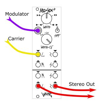
A classic patch from the LRMSMSLR, now perfected with the specifically designed VCA and 4QM through-zero stereo width processing circuitry of the MidSide+. Patch an oscillator to either the Left or Right input, set the Width control to Mono and then modulate with another Oscillator patched to the Width CV input. The modulation of stereo amplitude through zero will create very wide and thick sidebands in the stereo field
