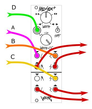
MidSide+ is DC coupled throughout, allowing for the processing of CVs as well as audio signals. MidSide+ can act as a collection of mixers, polarisers, a VCA, and a Four Quadrant Multiplier to combine simple CVs into much more complex and musically interesting combinations. Given four CVs (A, B, C, and D) patched to the Left (A), Right (B), and Side (C) Inputs, as well as the Width CV (D) input, the following combinations are created at the following outputs:
