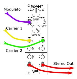
This is a variation of the Through-zero stereo ring mod patch above, with a third oscillator patched into the Right input. Make sure that there is some timbral difference and detuning between the oscillators patched to the Left and Right inputs, so that the Side signal being modulated morphs and breathes creating thicker moving sidebands. This technique excels at producing stereo drones, but also can create thick stereo
