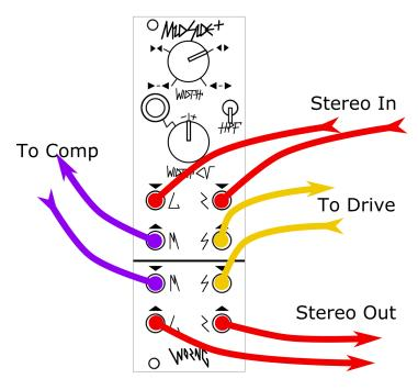
This is the basic functionality of MidSide+ and other Mid/Side processors, run your stereo mix into the Left and Right inputs and then use the Mid and Side processing loops to do symmetrical stereo processing of your signal using mono processors. A basic starting patch would be to run the Mid out to a compressor to create glue and energy in
