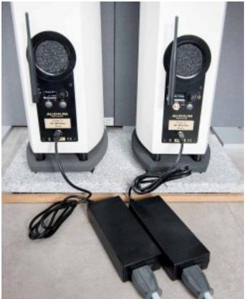
This pair of Audium Comp 5.2 AIR was already set up and the speakers were marked left and right. So I set them up directly like that and screwed the antennas on. The speaker position can be adjusted via the menu on the rear terminal of the speakers. The role of the master and the slave is technically predefined.
