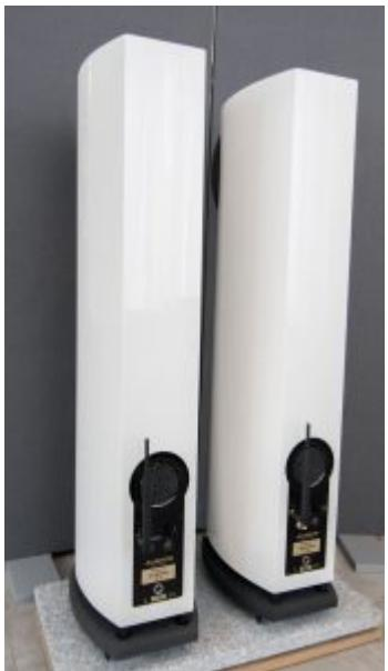
The rear user interface on the speaker with a rotary/push dial has a small graphical display. This helps to set speaker parameters such as room, bass boost, position as well as the tunable equalizer for easy, individual room adjustment. But also various other parameters such as display brightness, automatic switch-off, channel assignment etc. can be set.
