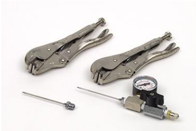
Manometer (Dual Track Welds)
