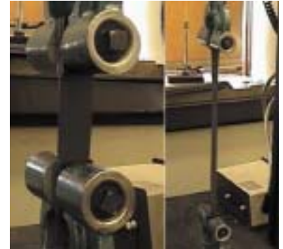
Photo 2: Exhumed PVC before and during tensile testing.
