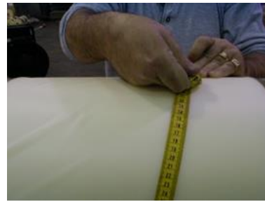
Figure 4: Incorrect Measurement because tape is not parallel to roll edge.
