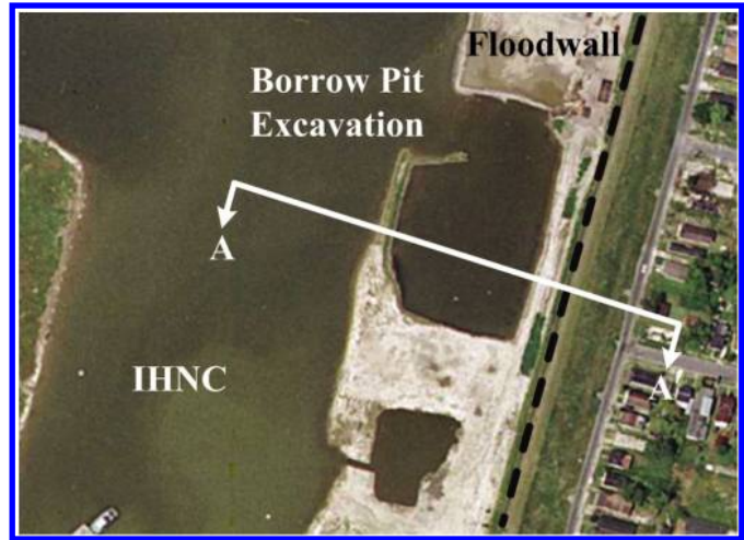
Fig. 3. Aerial view of large water-filled soil borrow pit excavation within 23 m of floodwall prior to Hurricane Katrina between north and south breaches ( 29^{\circ}58'41.50''N , 90^{\circ}01'14.14''W ; photo courtesy of Gulf Coast Aerial Mapping, Baton Rouge, Louisiana).
