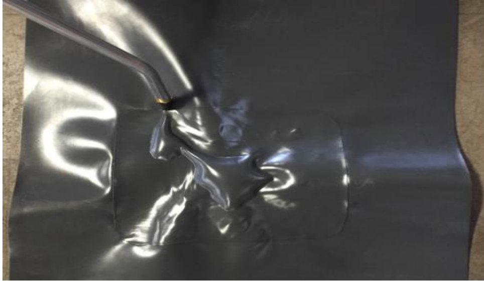
Figure 4: Performance of air lance test of a PVC patch that shows an aneurysm in the patch which means there is a leak.
