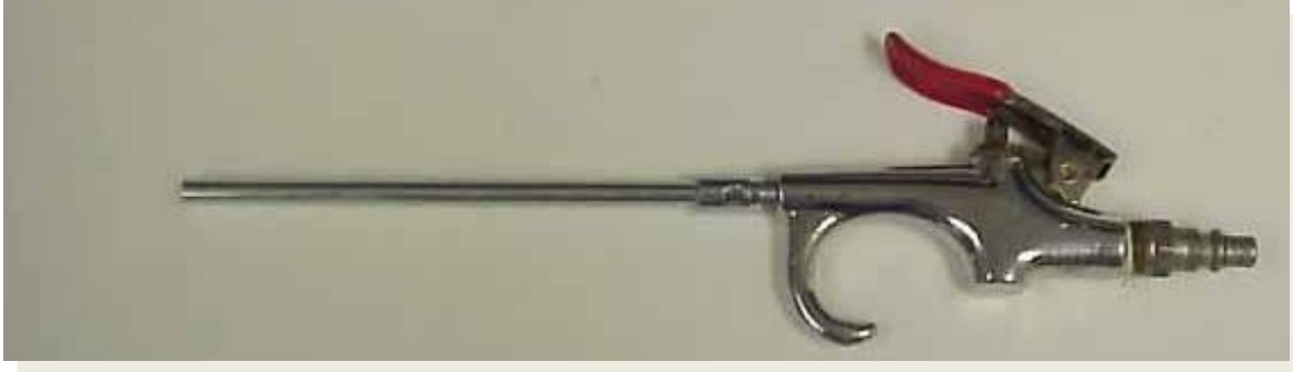
Figure 2: Air Lance equipment that attaches to air supply for testing
