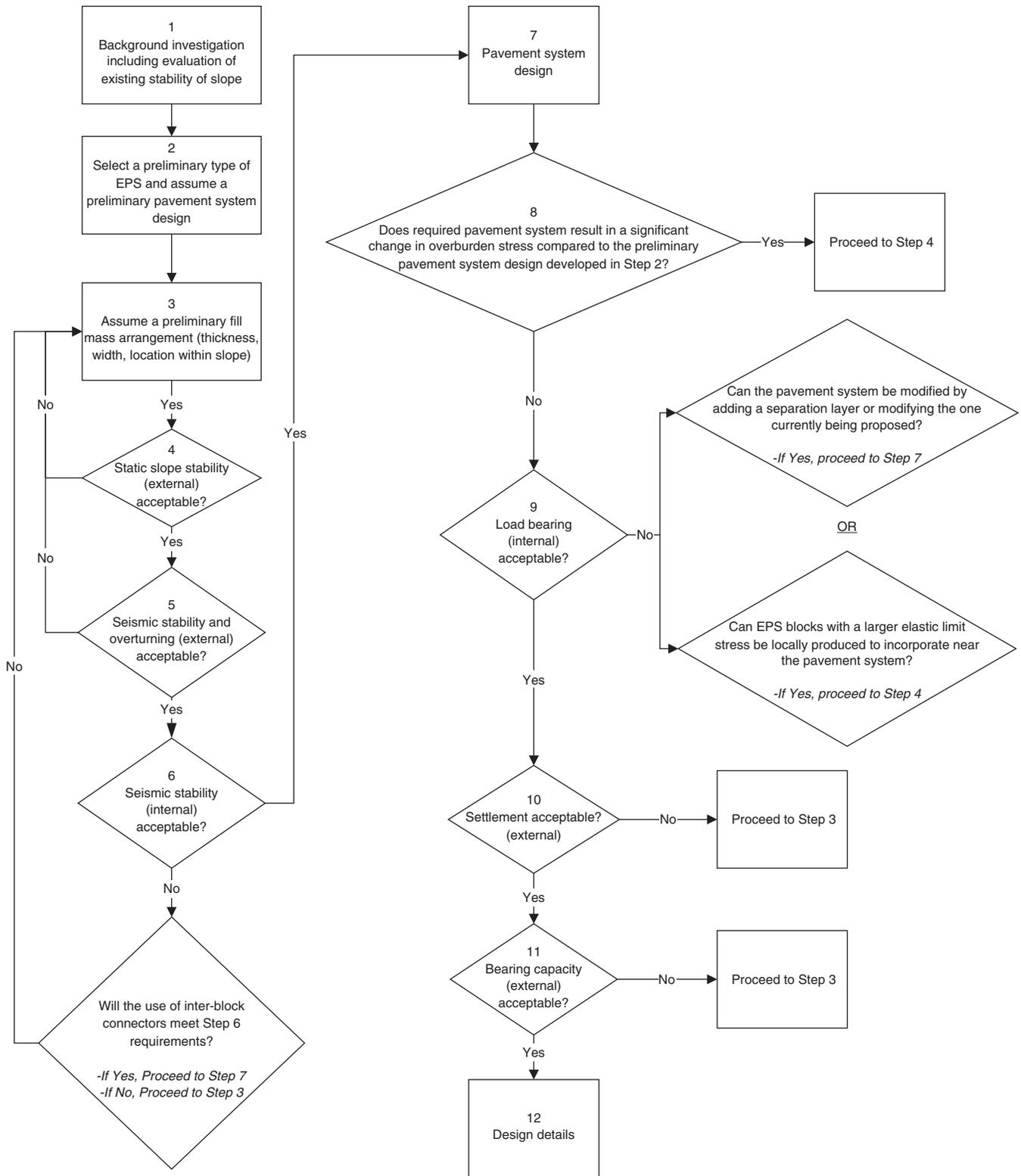
FIGURE 3 Recommended design procedure for existing or proposed roadway located within existing or anticipated slide mass and when existing or anticipated slide mass is located below roadway; that is, roadway is near head of slide mass.
