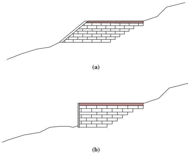
FIGURE 1 Typical EPS block geofore applications involving sidehill fills: (a) slope-sided fill and (b) vertical-sided fill (geofore wall).
