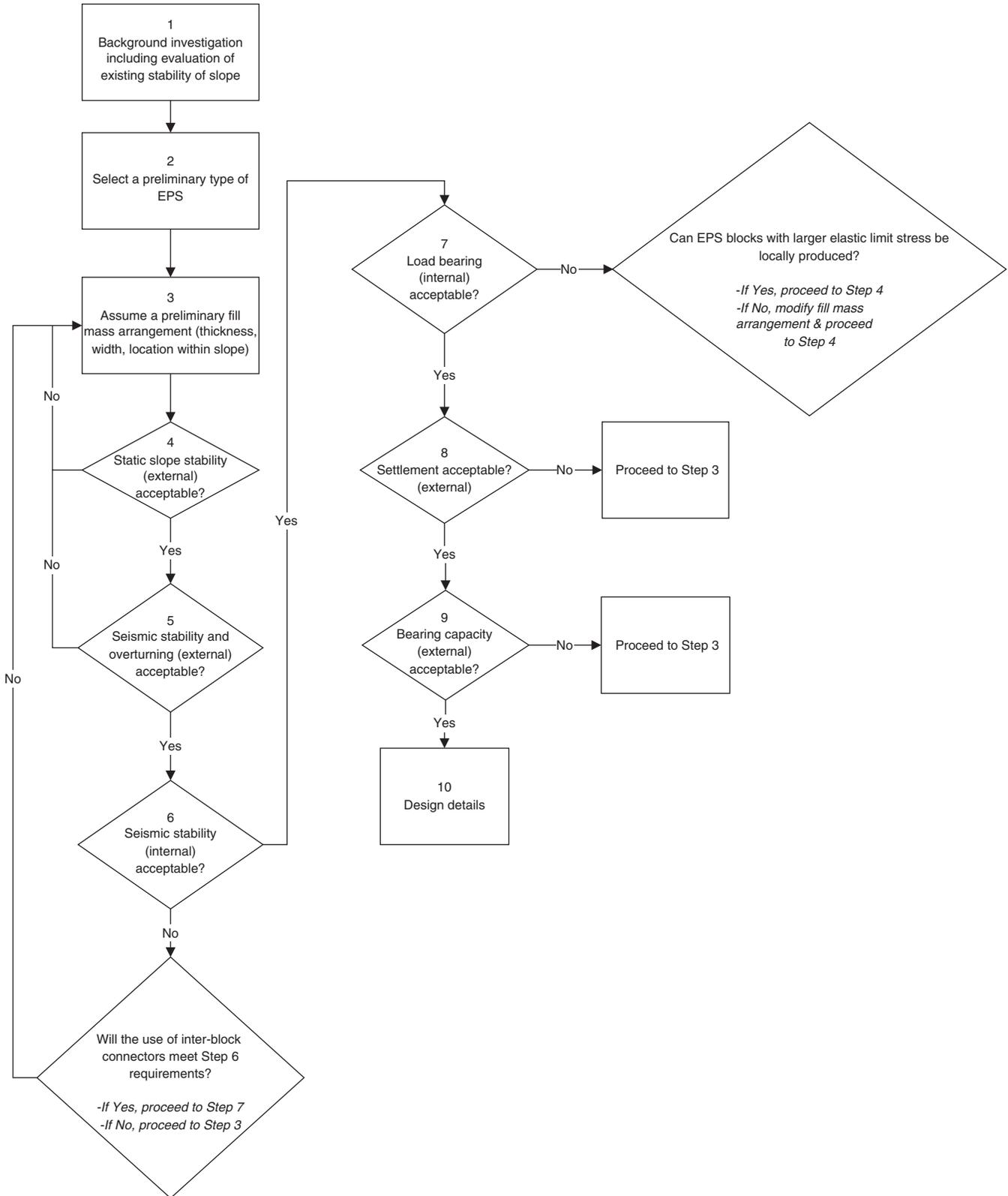
FIGURE 4 Modified design selection procedure for existing or proposed roadway located outside limits of existing or anticipated slide mass, when existing or anticipated slide mass is located above roadway, or both; that is, roadway is near toe of slide mass.
