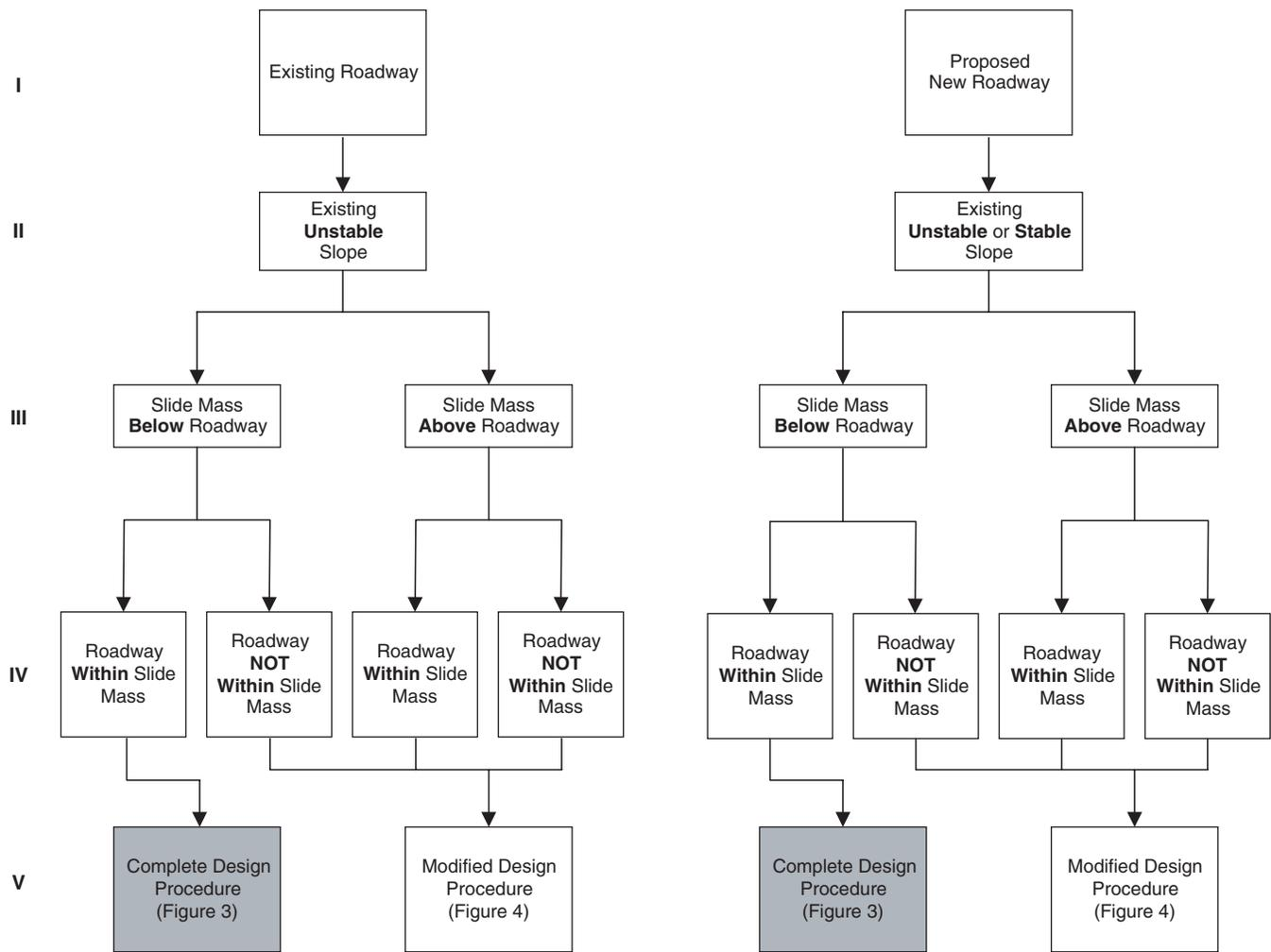
FIGURE 5 Design selection procedure diagram.
