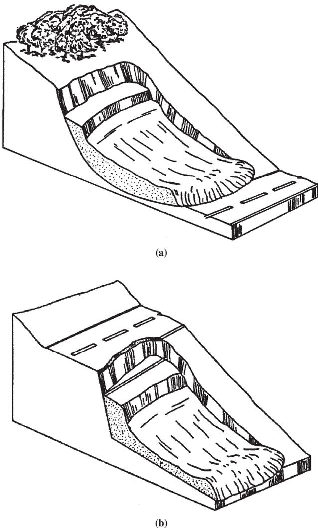
FIGURE 2 Location of slide mass relative to roadway: (a) slide above roadway and (b) slide below roadway (34).
