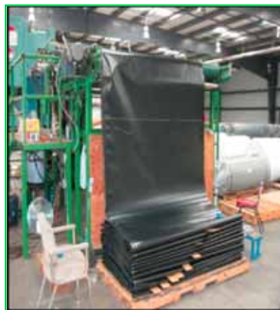
Folding of 30 mil. factory fabricated geomembrane panels.
