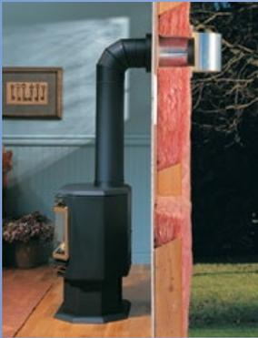
Direct vent technology means that you can install a Regency stove almost anywhere in your home - no chimney is needed. From the top of the unit, simply vent your stove through an exterior wall. Direct vent means that you have sealed combustion - outside air is brought in through the vent for combustion and the used air is sent back out - your indoor air is not affected.
