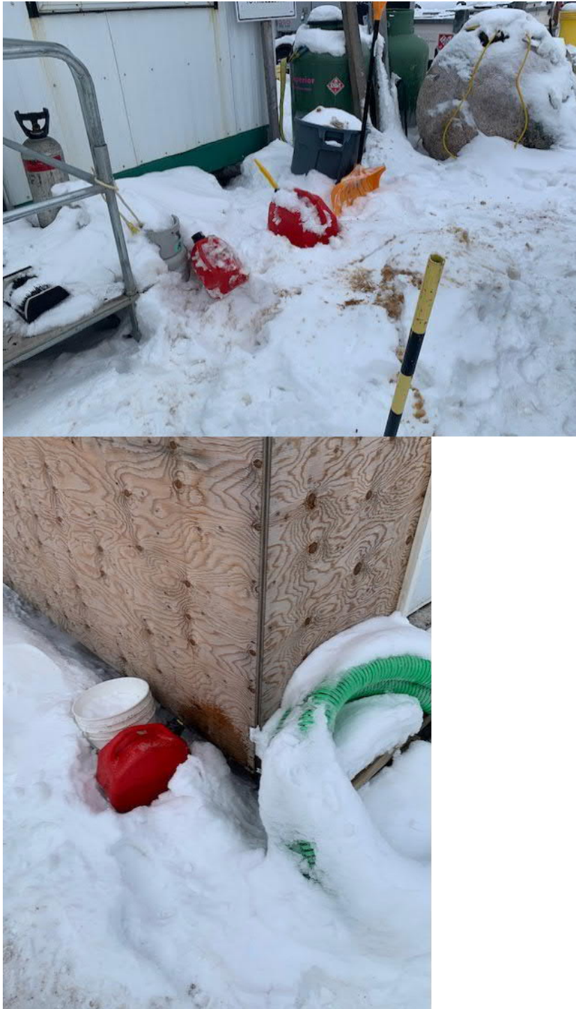
Photo 20: Junction Camp/Red Lake Yard – Jerricans missing secondary containment and labels.
