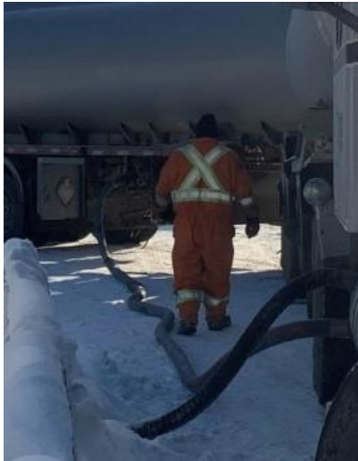
Photo 5: Sioux Lookout Camp and yard – Fuel truck (third party) came by and started refueling. No spill tray was used, missing PPE (glasses).
