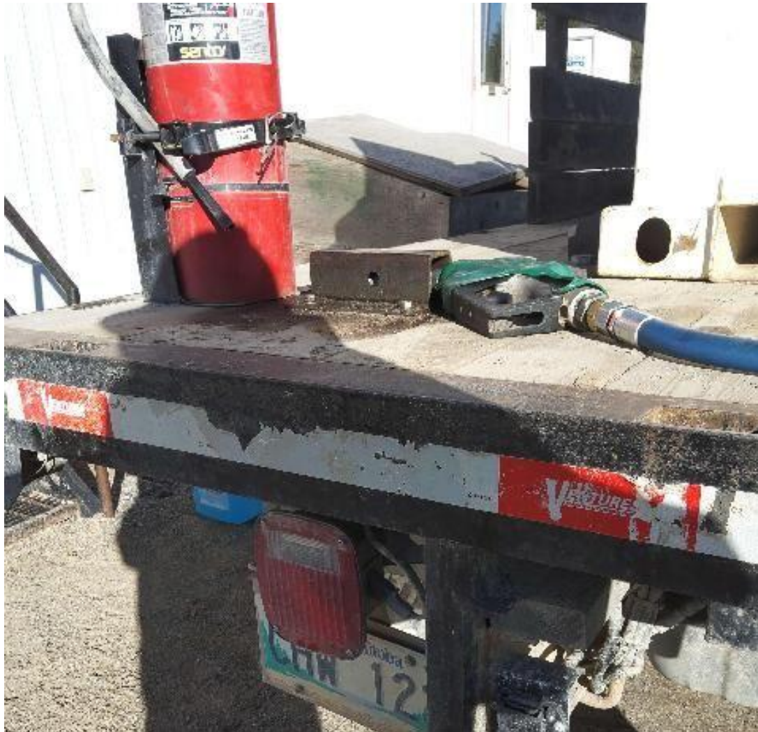
Figure 2: Nozzle for mobile fuel tank not properly stored
