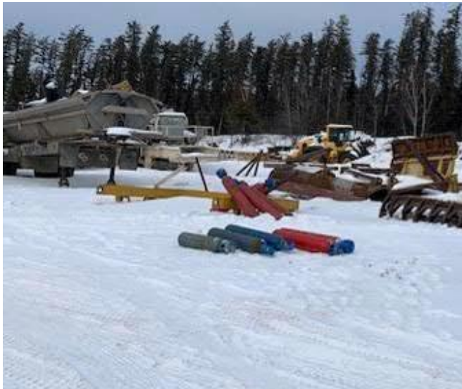
Photo 18: Junction Camp – Compressed gas cylinders not stored properly.
